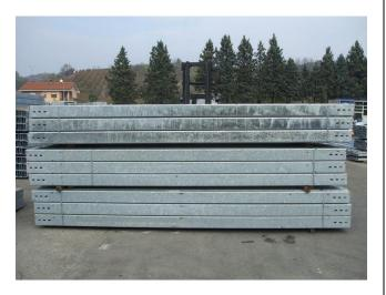
HANDLING AND STORAGE OF ROAD BARRIER UPPER BEAMS 26/03/2024
